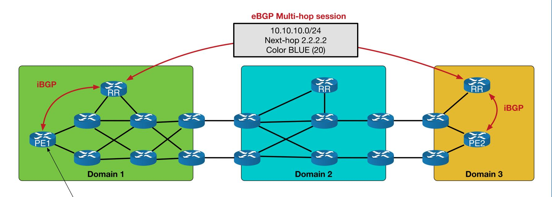
PE1 might not have an IP route to the next-hop (in this case 2.2.2.2). This could be provided using an aggregate route or less-specific null static that is redistributed.
